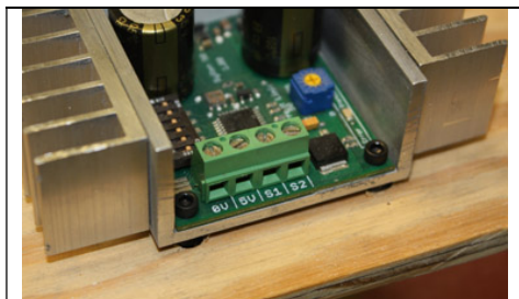
Figure 2.3: Mounted to a wood frame using standoffs
