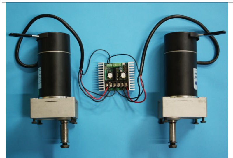
Power outputs connected to electromagnetic brakes.
